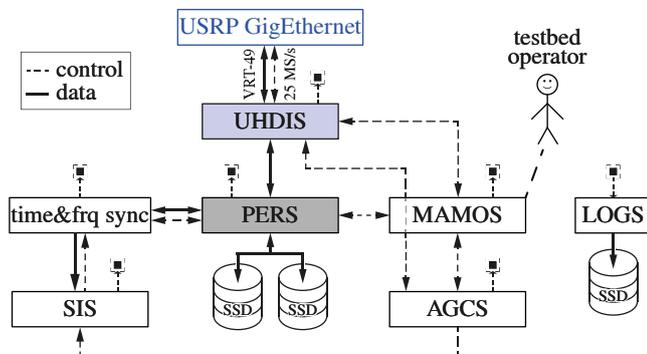
Fig. 3. High-level scheme of the low-level and real-time processing software. Note that all software modules are connected to "LOGS".
