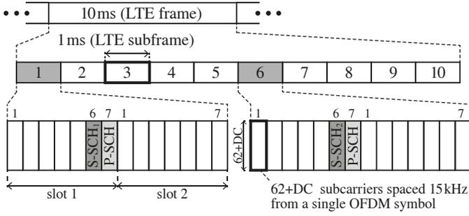
Fig. 4. LTE synchronization signals.
