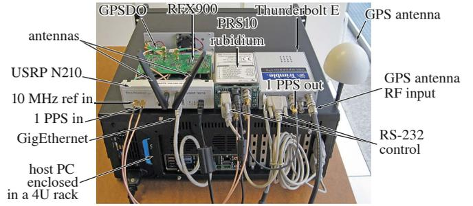
Fig. 1. Picture of a node from the testbed. Notice that all components appear outside the PC case but they perfectly fit inside it (except the antennas).
