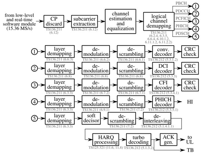
Fig. 6. Scheme of the implemented receiver software module.
