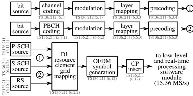
Fig. 5. Scheme of the implemented transmitter software module.
