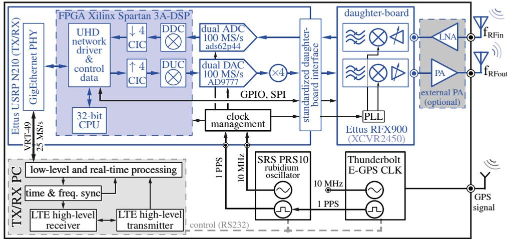
Fig. 2. Scheme of the testbed hardware consisting of a PC, a USRP N210 with the RFX900 RF daughter board and the GPS+Rubidium reference oscillators.
