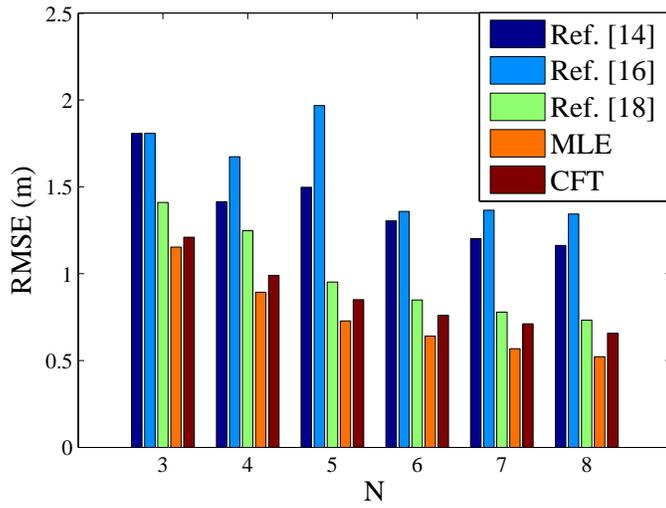
**Fig. 7** RMSE of the positioning error for different localization techniques as a function of the number of beacons, for the floor plan in Fig. 5
