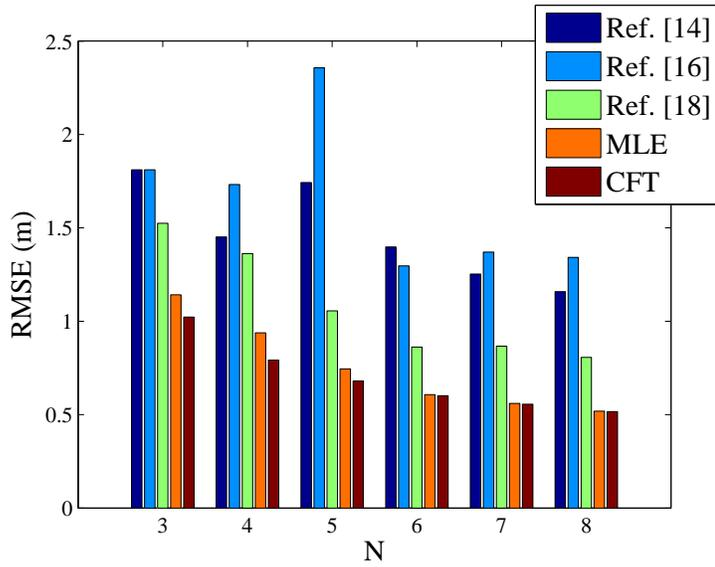
Fig. 4 RMSE of the positioning error for different localization techniques as a function of the number of beacons, for the floor plan in Fig. 1
