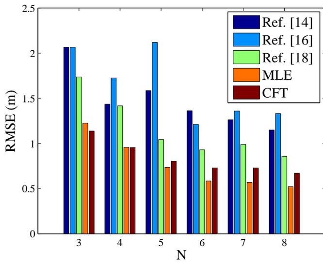
**Fig. 8** RMSE of the positioning error for different localization techniques as a function of the number of beacons, for the floor plan in Fig. 6
