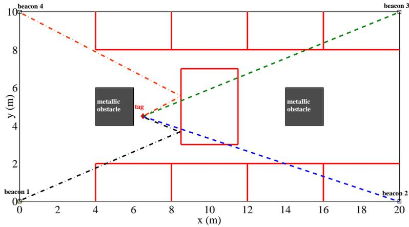
**Fig. 3** Trajectories corresponding to the shortest tag-beacon paths, for a tag situated at  $(6.5, 4.5)m$  in the floor plan of Fig. 1, with four beacons.
