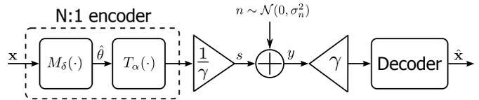
Fig. 1. Block diagram of a bandwidth compression  $N:1$  analog JSCC system over an AWGN channel.
