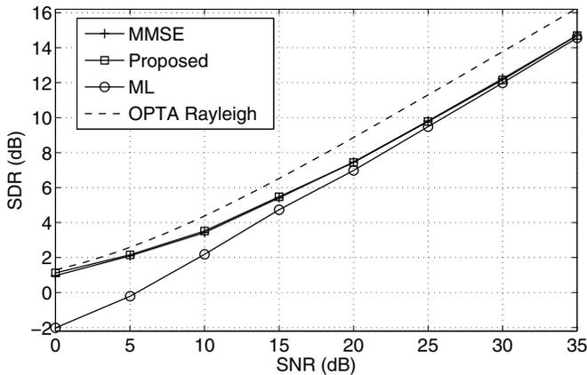
Fig. 3. Performance of the 2:1 analog JSCC system described in the text when a SISO Rayleigh fading channel is considered.
